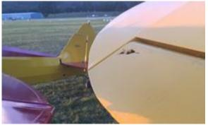
Aircraft wing tip was pushed into an aileron, poking a hole in a perfectly good flight control.
